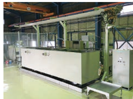
Penetration Inspection Pretreatment Device
