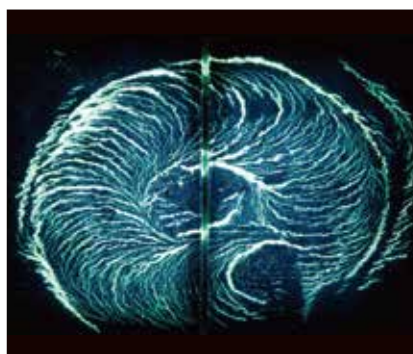
Type3: JIMA TP-03 (AL burning crack specimen)
